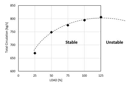
Figure 4. Total circulation of the boiler as a function of load
