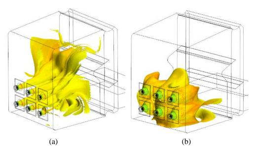
Figure 3: Isosurfaces of luminous flame contours for gas injectors oriented (a) toward the center, and (b) axially
