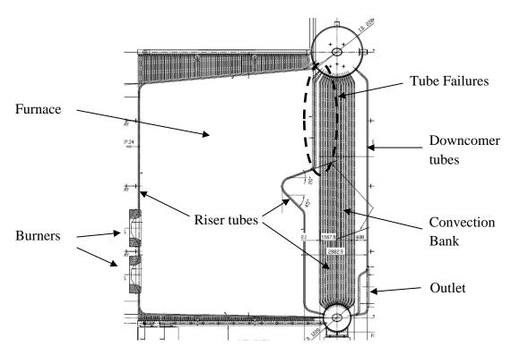
Figure 1. Schematic representation of a VU-60 Boiler
